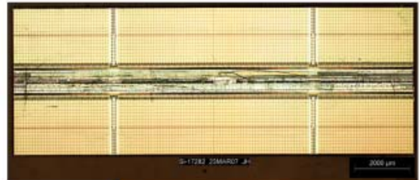
Die photo of Qimonda's 512-Mbit DDR3, which, at 14.6 x 5.4 mm, is more of a rectangle than the squarish DDR2.
