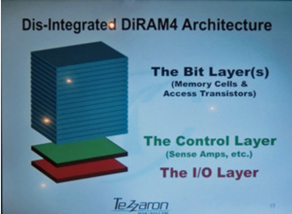
16 pieces of memory chips and control layer, examples of stacking chips of the I/O layer
